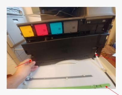
Take the Green Rod off of the front door, and insert it into the 4 process unit housings.
