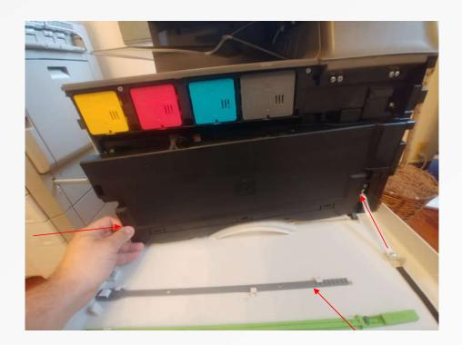
Insert the Gray rod with the Cloth Pad First, Facing downward. The pad cleans to Laser glass. Run the Gray rod Through all 4 Laser Glasses as shown below.
