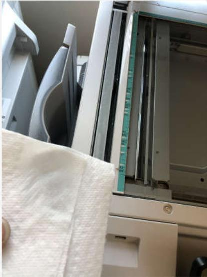
Then wipe the small strip of glass on the left of the Platen glass until you can no longer see any dust, ink or white out.
