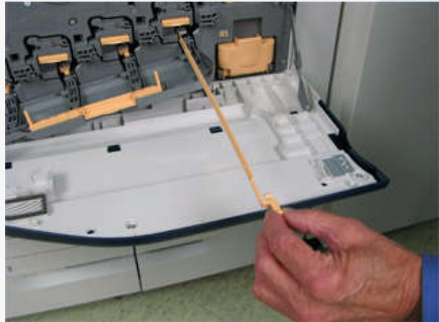
After pushing the rods back in, close the drum door and rotate the orange lever back to the right. You can now close the door and try your print job again. The color dropout should now be gone. If it isn't, move to the next slide.
