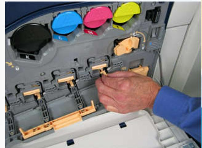
Gently pull the cleaning rod out until it stops. It does not come out of the machine. Do this for each of the colors twice. This will clean any dust or toner off of the machines print heads.
