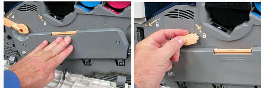
If you still see a drop in one of the colors in your picture, and you can see that it is one specific color, try swapping that color's drum with the one next to it. All of the drums can be swapped with each other. Carefully remove the drum and set aside. Then move the next drum over to the empty slot. Re-insert the drum into the machine and test print. If the color dropout moves to the color you swapped with, replace that drum with a new one. This should fix dropouts in your color prints.
